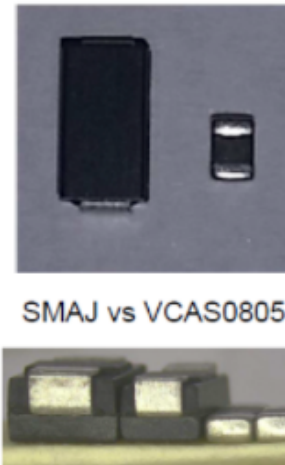
Figure 3: Replacing a SMAJ TVS with a 0805 size varistor. Image courtesy of KYOCERA AVX
