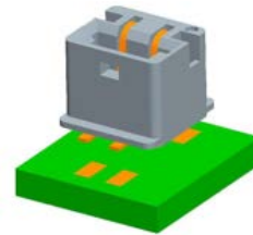
Connector drops straight onto PCB
